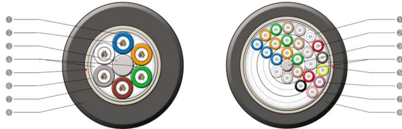
① Loose Tube ② Optical fibers ③ Central strength member ④ Core filling ⑤ Ripcord ⑥ Core wrapping tape ⑦ Outer strength member ⑧ Outer PE jacket
